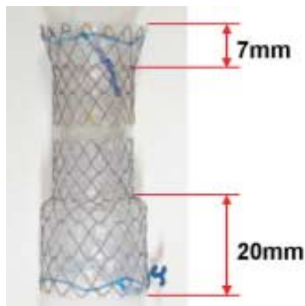
Figure 1 Newly designed self-expanding metal stent (SEMS) for the cervical esophagus. In order to decrease the foreign body sensation and to prevent migration of the stent, we reduced the length of the proximal funnel to 7 mm. The expanded diameter is 18 mm.
